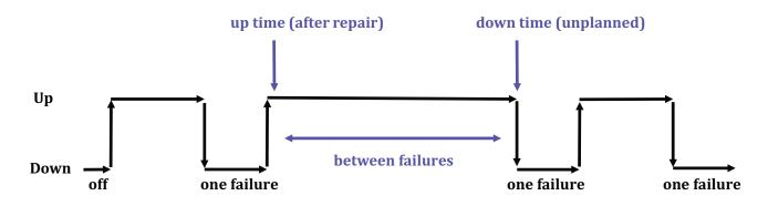
Time Between Failures = { down time - up time }
